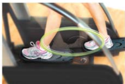
MEASURING MOTION CR engineers trace the pattern of elliptical pedals as they turn to help assess the ergonomics, from heel to toe.
